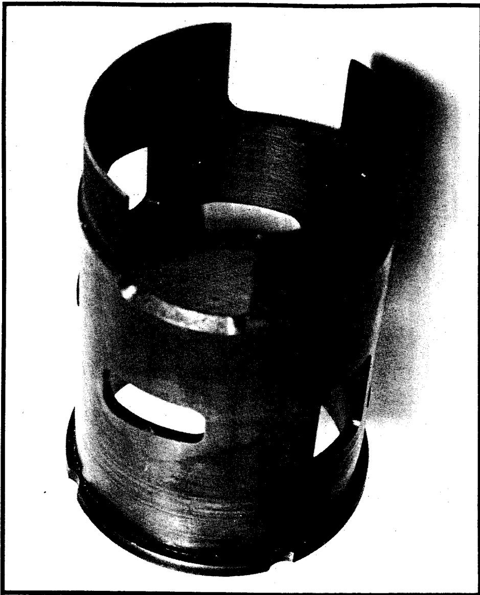
Bevelling the edge of the transfer ports produced better scavenging, more low-rpm power.
